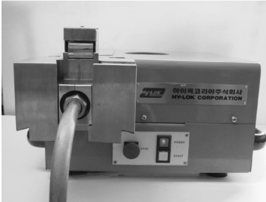
Overall dimensions : 400 x 400 x 230. Weight : 50 Kg.
